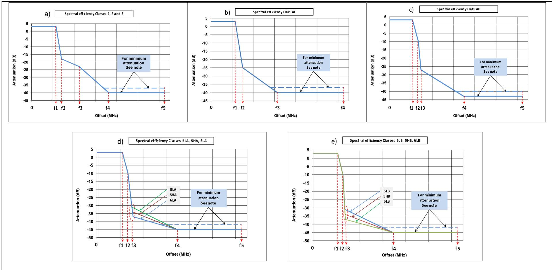
NOTE: The noise floor attenuation depends on the CS; see table 2k for details.
