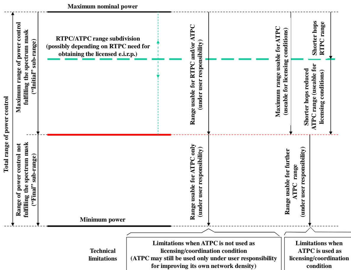
Figure I.1: ATPC/RTPC ranges and licensing/coordination conditions
