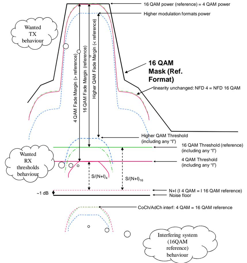
Figure I.3: Example of nodal co-channel interference (reference modulation format 16QAM):
